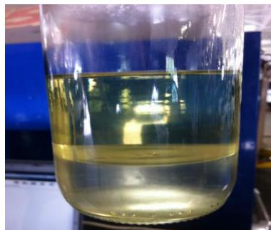
Slops is the fuel drained off to perform samples and quality control tests that cannot be returned
